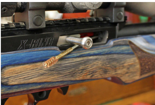
Feed the cable through the ejection port.
