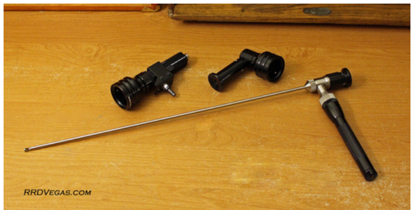
Borescope, Sony camera, and angled eye piece.
