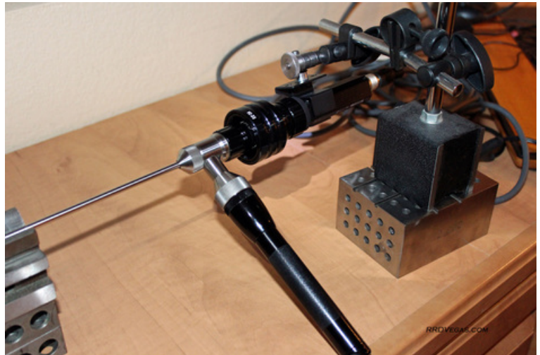
Sony camera hooked up to the borescope.
