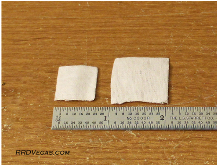
Proper patch size ( Left ) for cleaning the 0.17" bore.
